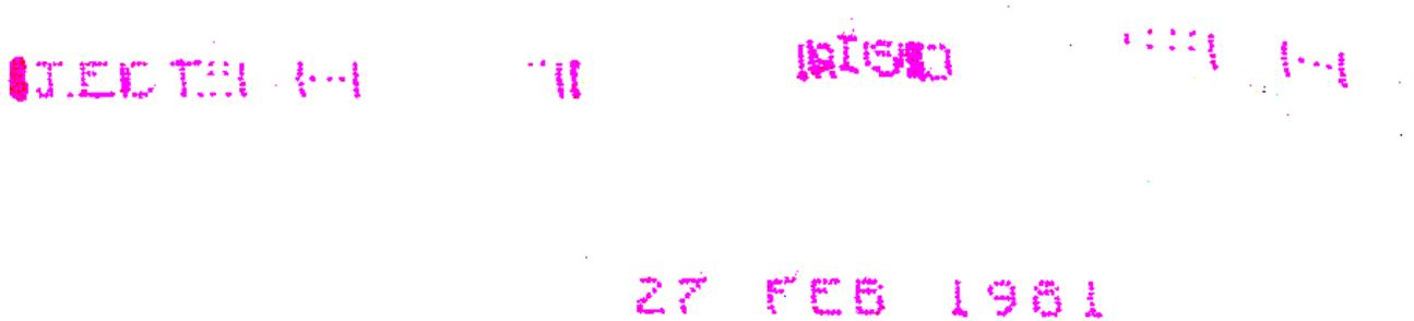
(First dot matrix text message printed with a thermal inkjet printhead in Corvallis)
