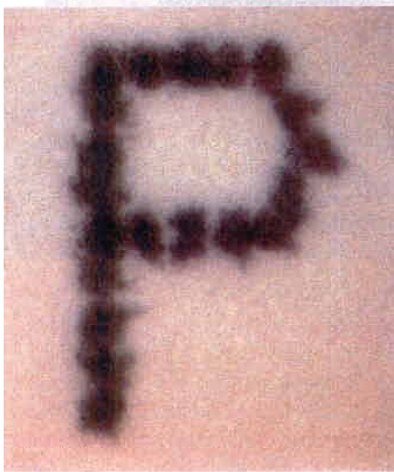
The 1984 ThinkJet, Hewlett-Packard's first inkjet printer (seen at top left), printed at 96 dots per inch, leaving a noticeably fuzzy outline.
