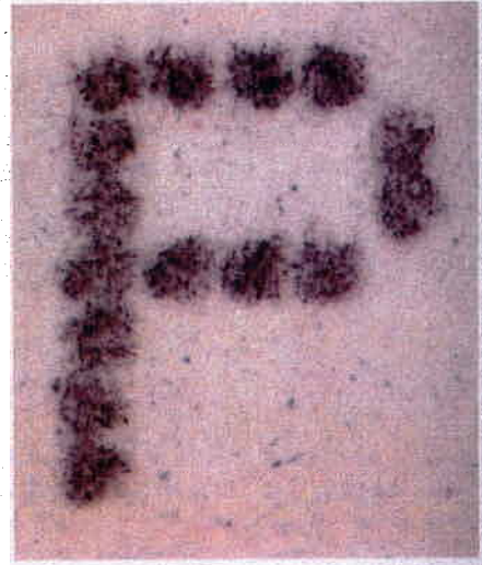
An early dot-matrix printer achieves only 80 dots per inch, and the dots are much darker on the "hilltops" of the microscopically rough paper surface.
