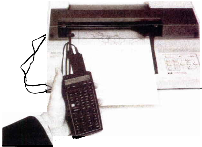
The X-Y plotter, an ancestor of the inkjet printer, used a grit wheel to move the paper along one axis while a felt-tip pen was driven back and forth along the other.
