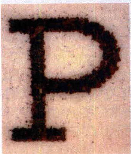
The 1988 DeskJet printed 300 dots per inch and used a specially formulated ink that allowed smaller drops, which resulted in more precise characters.
