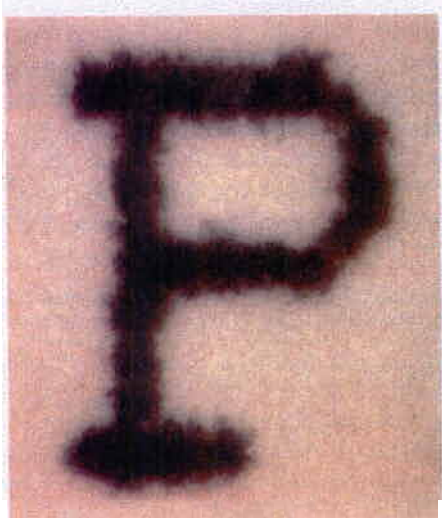
By making a second pass, Hewlett-Packard's 1985-86 QuietJet could print 192 dots per inch. Drop size would later be reduced for better results.
