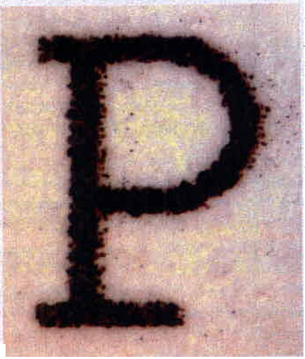
By 1995 the DeskJet 800 was up to 600 dots per inch and shot out droplets one-sixth the volume of those used in the ThinkJet of a decade before.
